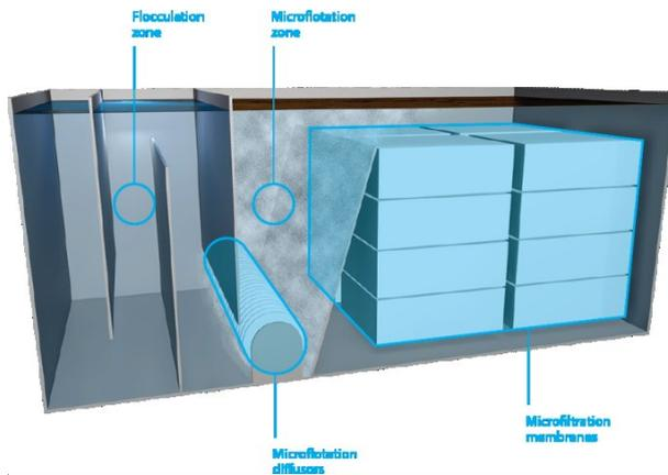
The microflotation process of the akvoFloat™
