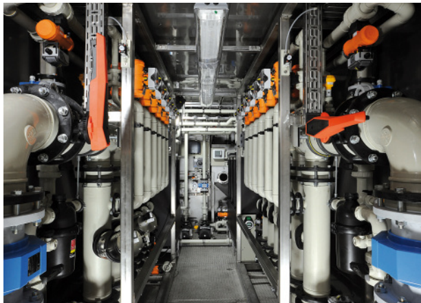
Redundant ultrafiltration modules inside of OilPaq container for fracking flowback and produced water treatment (Photo: Business Wire)
